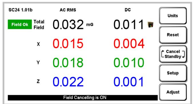
Fig. 2. Typical touch screen display with DC sensors
