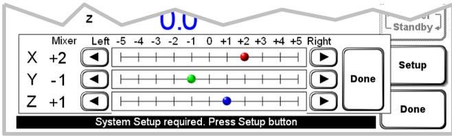
The “Mixer” button opens a sub-screen with sliders to adjust the mixers, shown above. Run “setup” after adjusting the mixers (recommended).
