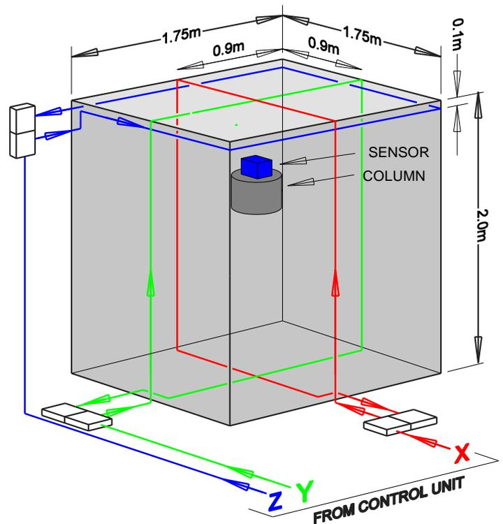
Fig. 5. Minimal Installation
