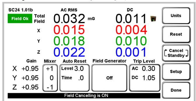
“Setup” automatically sets the feedback loop gains and phases. The gain values are displayed for reference. There is no manual adjustment.
