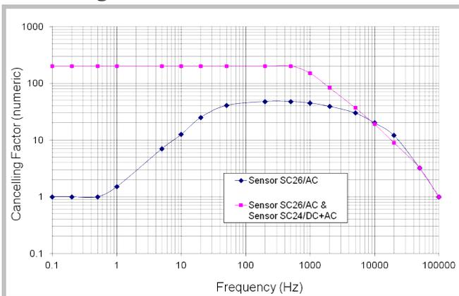
The “cancelling factor” is the ratio of the ambient field to the cancelled field. A graph of cancelling factor vs. frequency is above.
