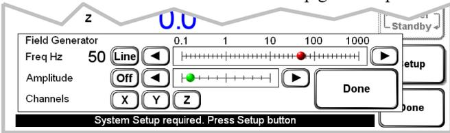
The field generator can be used to make fields and test the sensitivity of the electron beam tool to those fields. The fields can be sine wave at line frequency or square wave at the frequency selected using the sliders below. Square waves are low pass filtered at 11 kHz. The test field can be connected to the selected axes.
